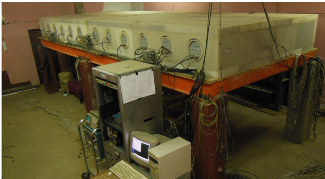
Figura 4: Monitor de Neutrones 12NM64
